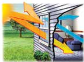
In summer months, Low-E glass helps block unwanted solar heat penetration to help conserve air-conditioning use.
