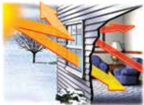
In winter months, Low-E insulating glass reduces heat loss by reflecting warmth back into your home.
