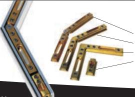
These clips nest into the top channel of the 4101A header. Use these clips to connect mitered header corners and to secure the header to the wall.
